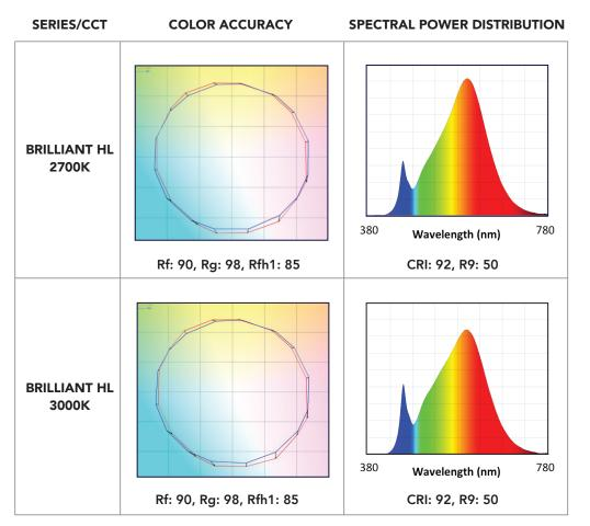
Rf: TM-30 metric measuring color fidelity (whether colors are similar to those under natural light). Rf is a more accurate version of the CRI Ra. Rf is 100 for natural light. Rg: TM-30 metric measuring color gamut (whether colors are more saturated than under natural light). Rg is 100 for natural light.
